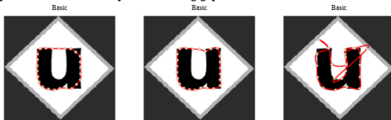
Figure 3.7: Result of the basic snake on a test image with \beta = 1 (left), \beta = 0.5 (middle) and \beta = 0 (right).
